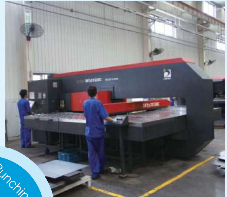
▼ SKYY31530C-type CNC turret pressure machine
