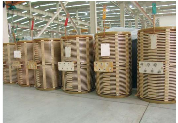
▲ HV H-class insulation winding
