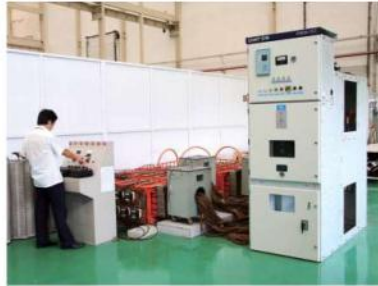
Power frequency withstand voltage testing platform ▲ ▲ Temperature rise test
