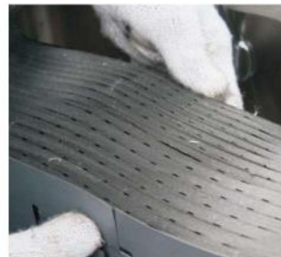
▲ Amorphous alloy core cross section
