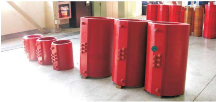
▲ F-class insulation HV winding
