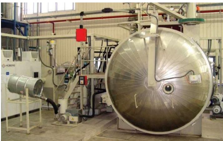
▲ Vacuum casting equipment from Germany HÜBERS adopts patented technology such as film defoaming and static mixer, ensure the transformer low partial discharge .
