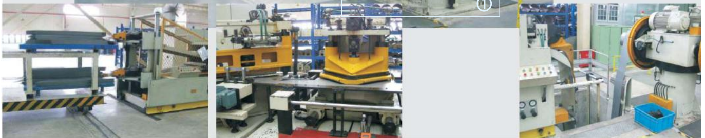
▲ ③ Automatically stacked silicon steel sheets ▲ ② Silicon steel sheet cutting
