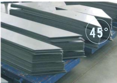
▲ The silicon steel sheet folded
