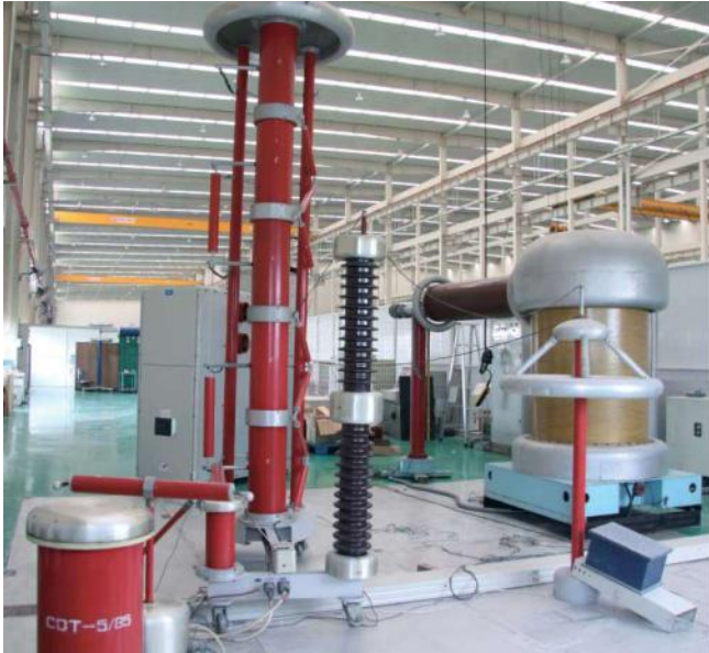
Lightning impulse testing platform ▲
