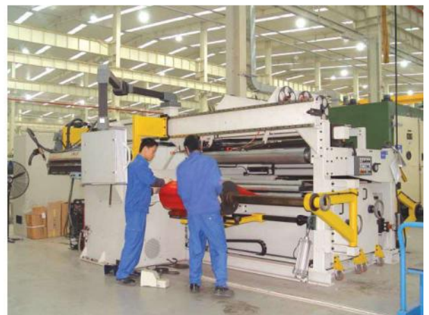
▲ TUBOLY LV foil winding machine from Switzerland which with constant tension, deburring, automatic bypass system and the corrective function
