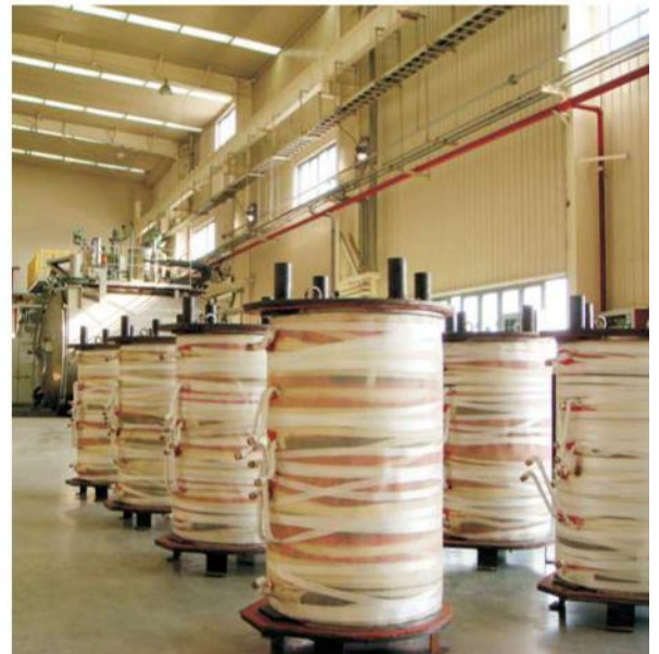
▲ HV F-class insulation windings before casting
