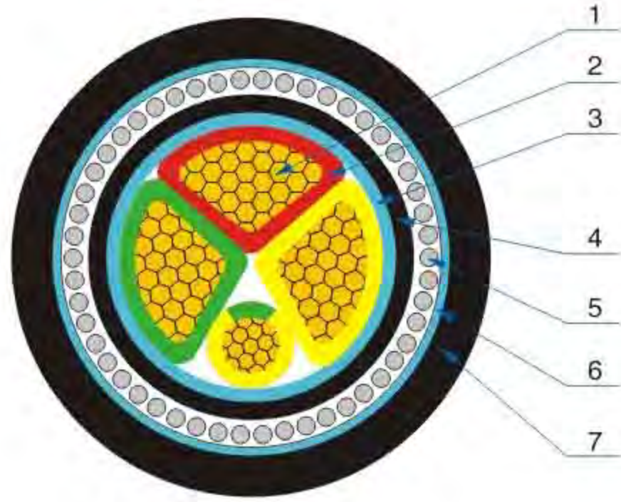
1-Conductor 2-Insulation 3-Binder tape 4-Inner sheath 5-SWA 6-Binder tape 7-Outer sheath
